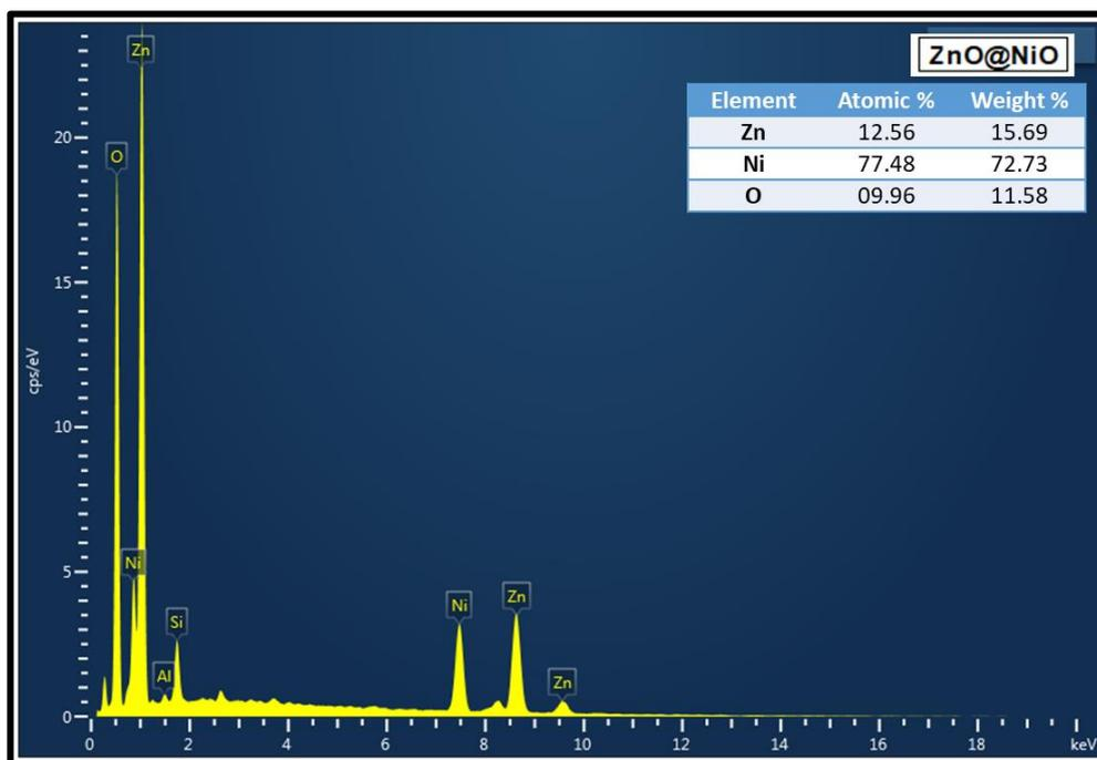
**Fig. 2.** EDX spectrum of ZnO@NiO nanocomposite
