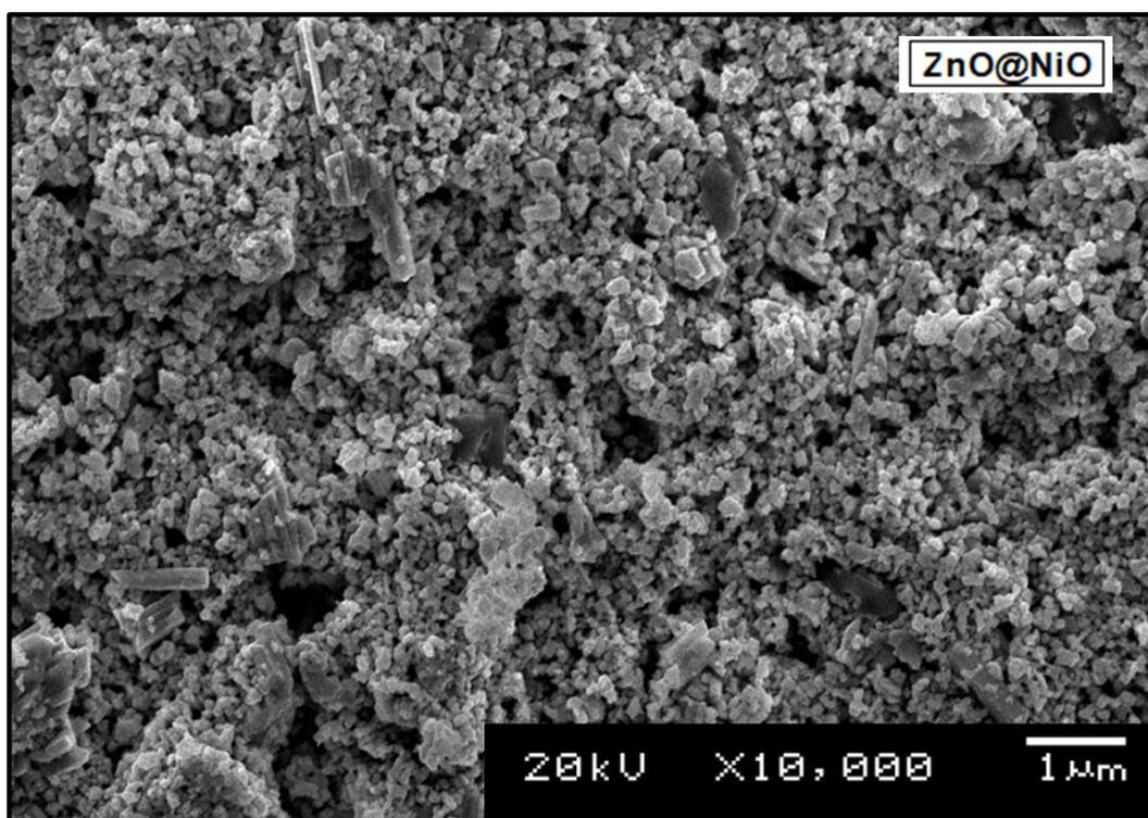
**Fig. 1.** SEM micrograph of ZnO@NiO nanocomposite
