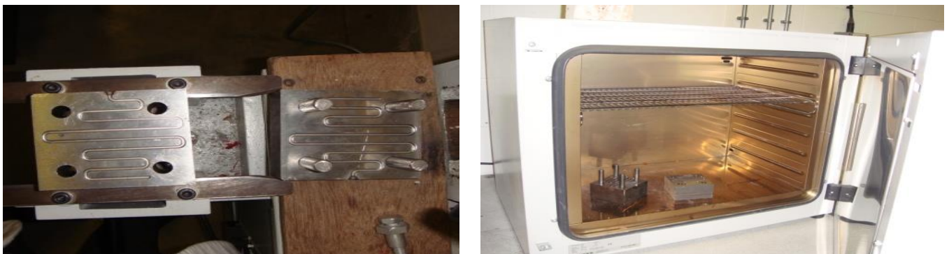
Fig 5: The Mould Form in the Furnace
