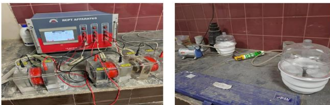
Fig. No.7. RCPT (Rapid Chloride Permeability Test)- ASTM C 1202
