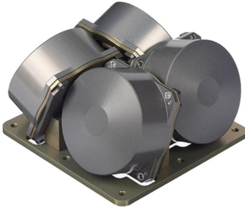
Figure 2. Tetrahedral reaction wheels of FLP [22].
