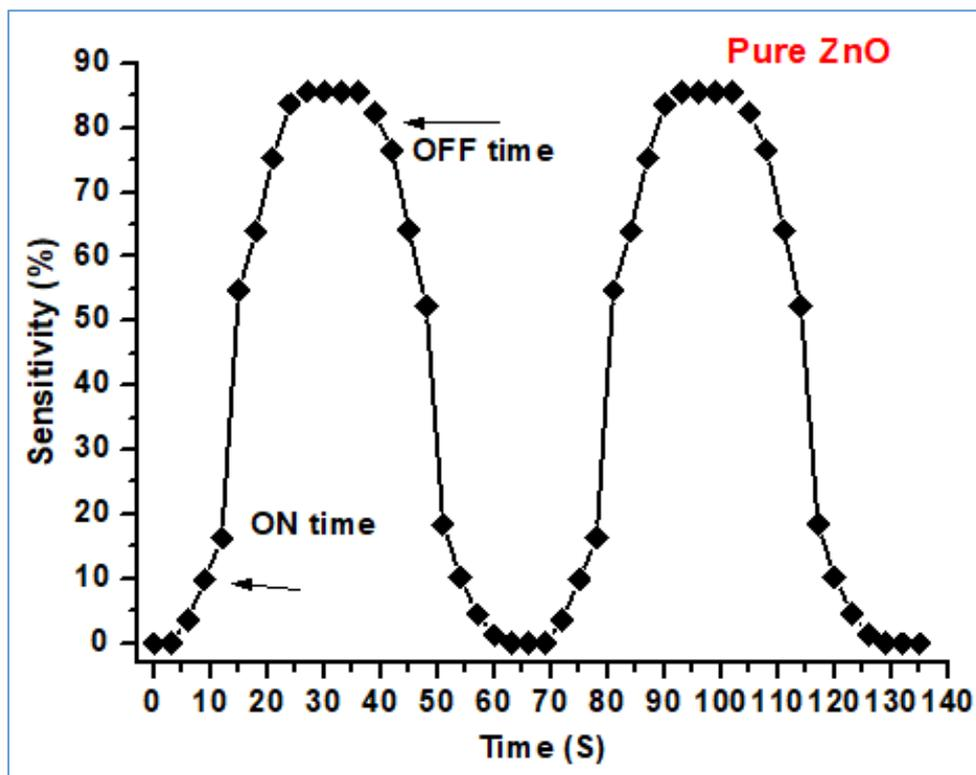
**Fig. 5.**Response and recovery time plot of ZnO thin films to LPG
