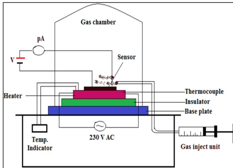
Fig. 1. Schematic diagram of static gas sensing system
