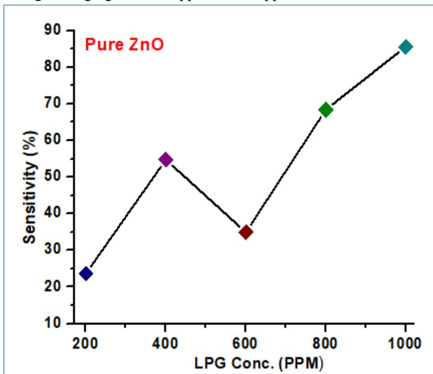
Fig. 4. Sensitivity versus LPG gas concentration (ppm) plot of ZnO thin films
