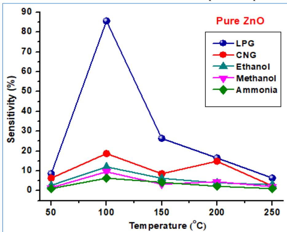
Fig. 2. Sensitivity versus operating temperature plot of ZnO thin films
