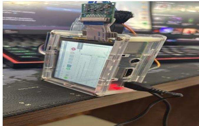
Fig 3. a Raspberry Pi-based wearable device encased in a transparent shell
