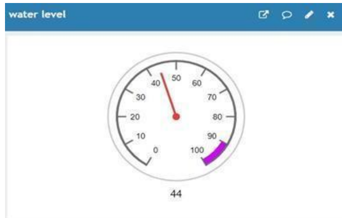
Fig. 7. Guage representation of fluid levels
