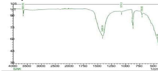
Fig .2 FTIR spectrum for calcium oxide nanoparticles
