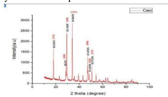
Fig.1 XRD spectrum for calcium oxide nanoparticle
