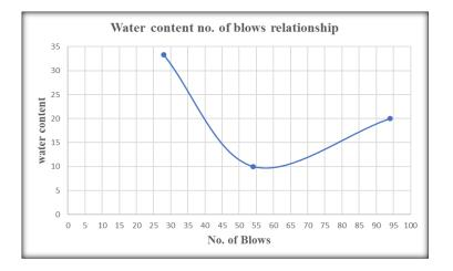
Conclusion – The liquid limit of soil is 34% and the soil has low plasticity .
