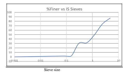
Conclusion – As Cu > 6 and Cc in between 1 and 3 the above black cotton soil is well graded sand
