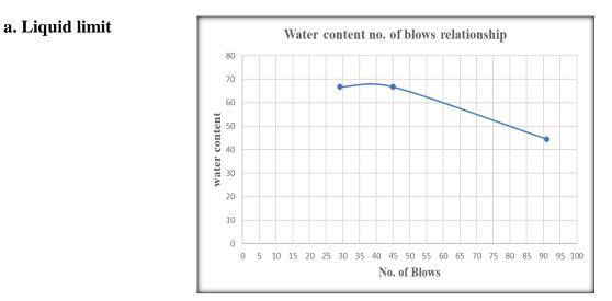
Conclusion – The liquid limit of soil is 66.6% and the soil has high plasticity.
