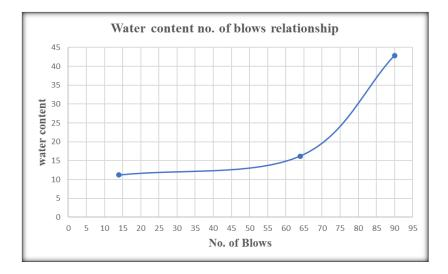
Conclusion – The liquid limit of soil is 38% and the soil has intermediate plasticity.
