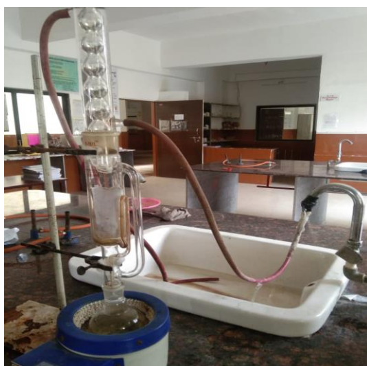
Fig: 5 soxhlet Apparatus Assembly
