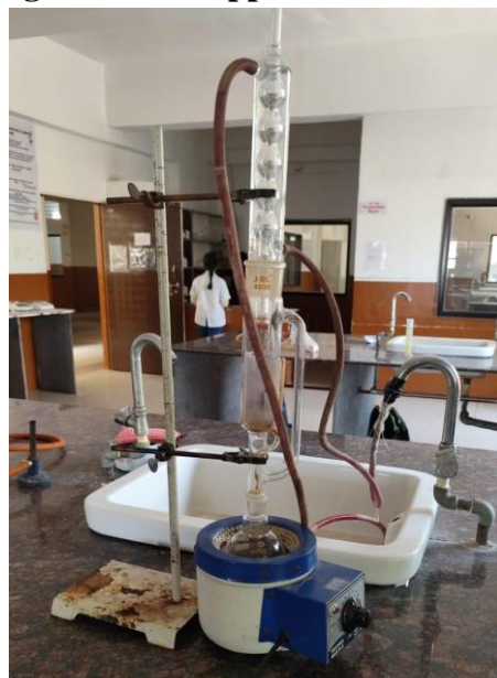
Fig: 5 soxhlet Apparatus Assembly
