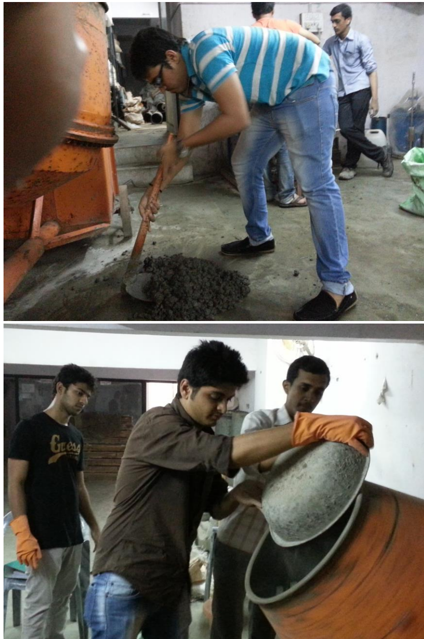
Figure 4.1: Mixing Of Rice Husk Ash (RHA) Concrete By Hand Mixing
