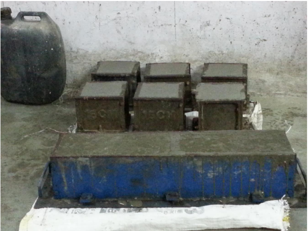
Figure 4.2: Casted Beams And Cubes
