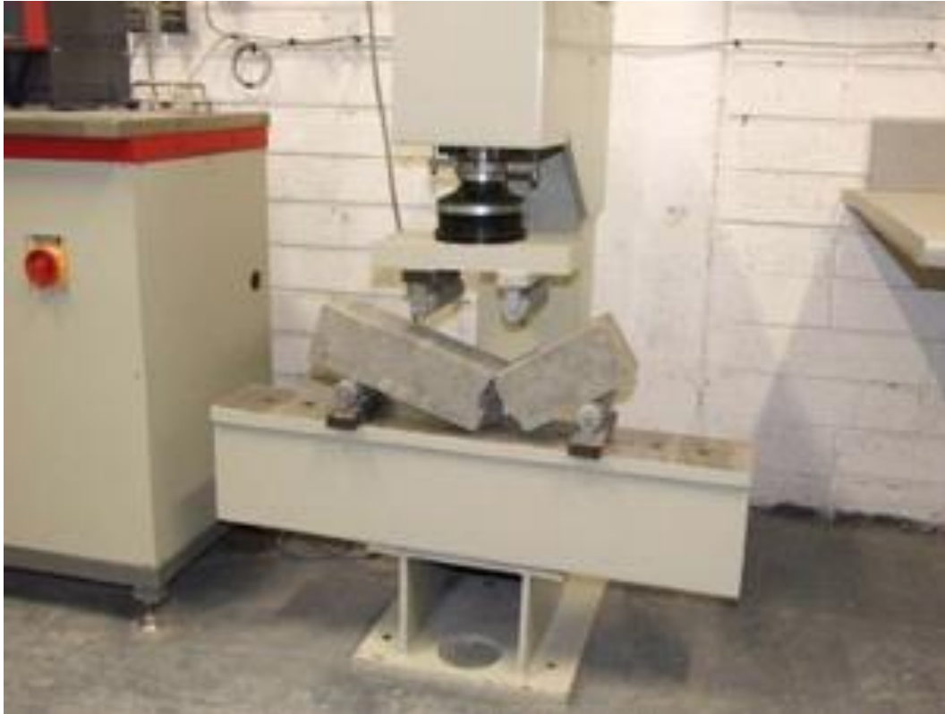
Figure 4.5: Flexure Strength Machine
