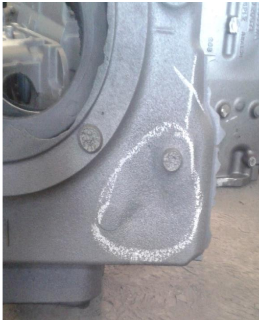
Fig.4.2-Shrinkage defect in casting
