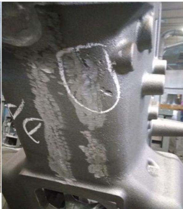
Fig.4.3.Sand Inclusion in casting.
