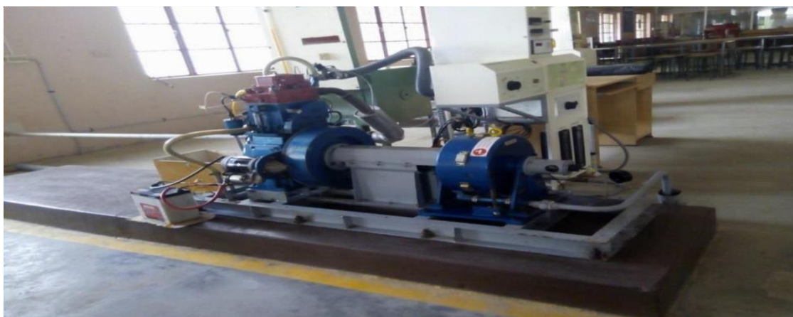
Figure Experimental Setup of VCR Diesel Engine
