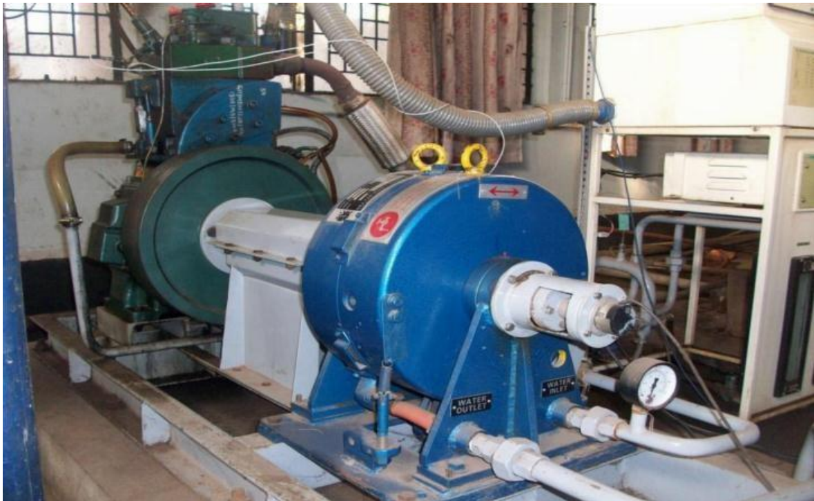
Assembly of Eddy Current Dynamometer and Engine
