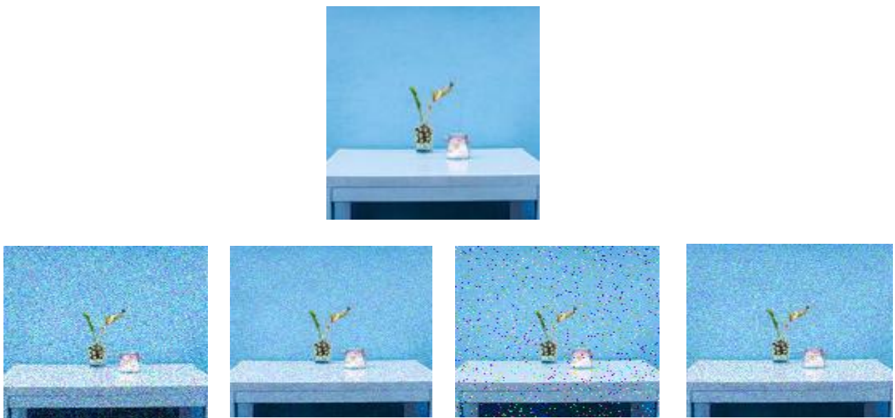
Figure 1: Sample dataset images depicting Ground Truth (clean image), Gaussian Noise, Poisson Noise, Salt & Pepper Noise, and Speckle Noise.
