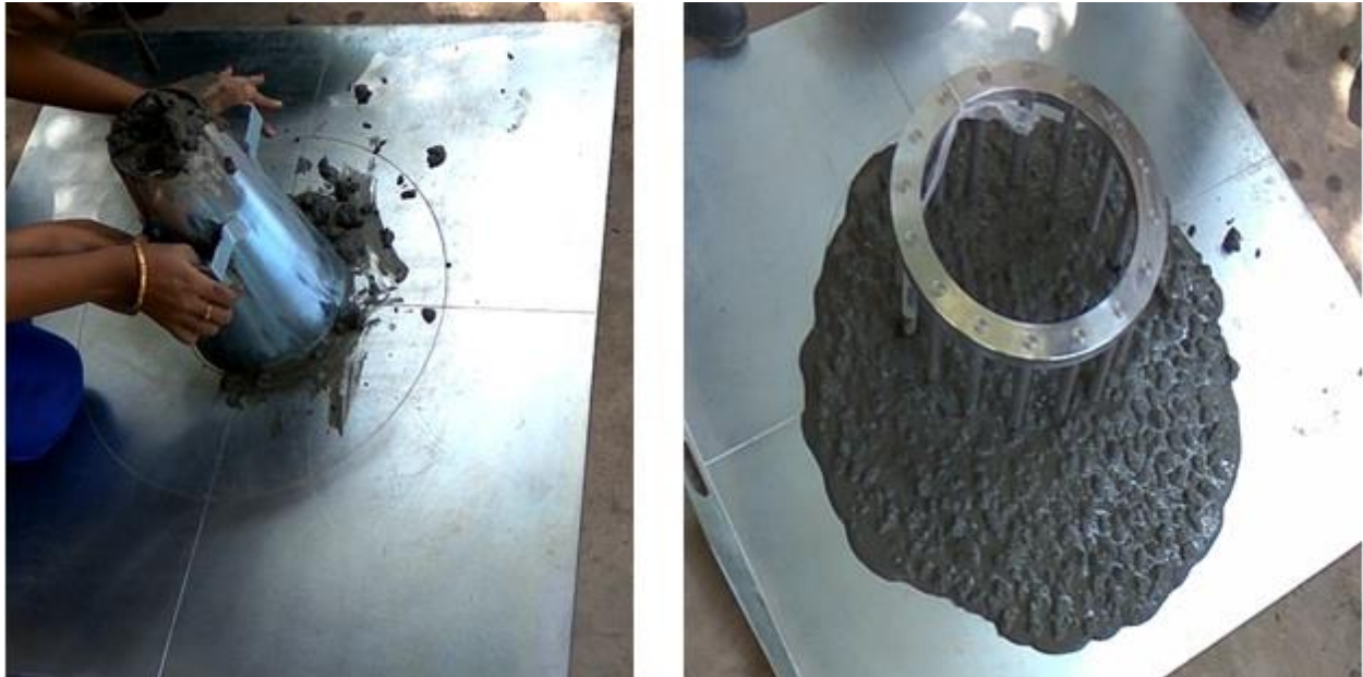
Figure 5: Progress of the J-Ring test.
