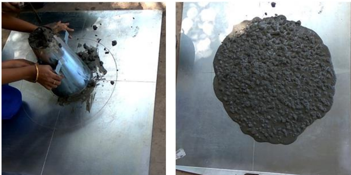
Fig. 4 - Progress of slump flow test
