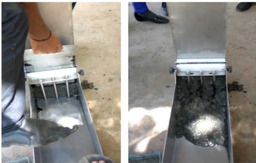
Fig. 7: Progress of L-box test.
