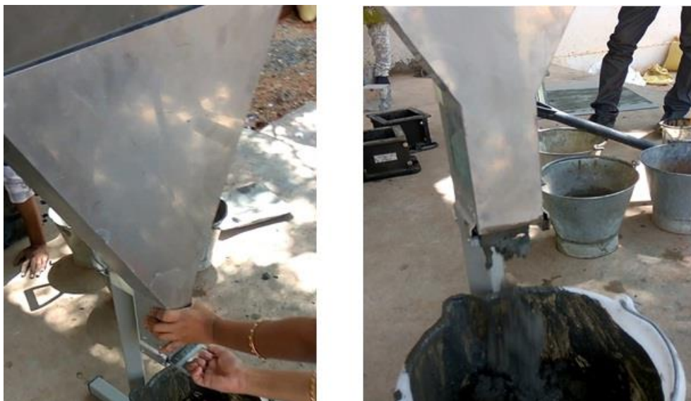
Figure 6: Progress of V Funnel Test.
