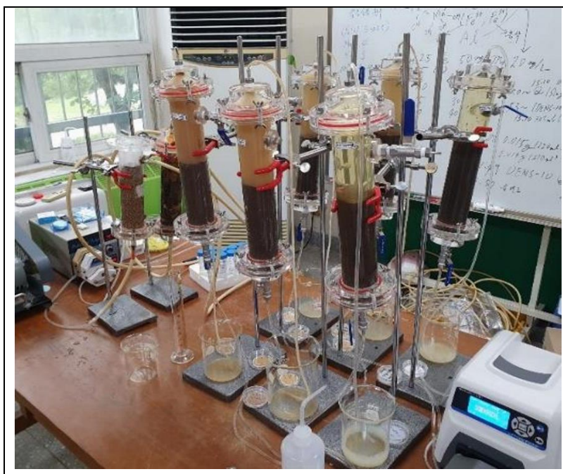
Figure 3: Column leaching setup for long-term evaluation of Pb leachability.
