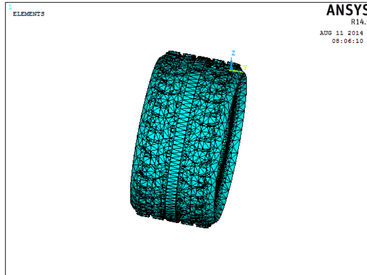
Fig 6.2 Meshed model of Skoda car tyre part
