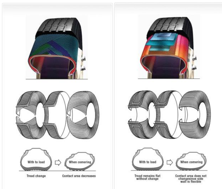
Fig:1.4 Schematic representation of Tyre Structure
