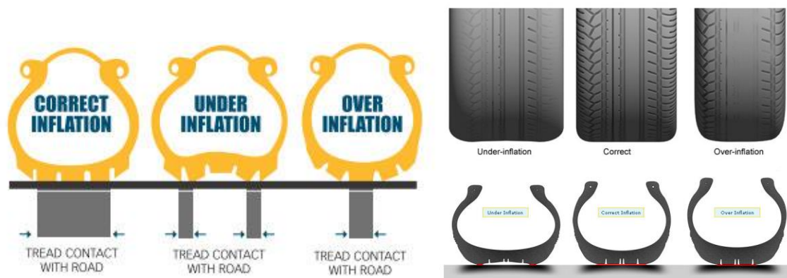
Fig:1.3 Tyre variations based on Inflation Pressure
