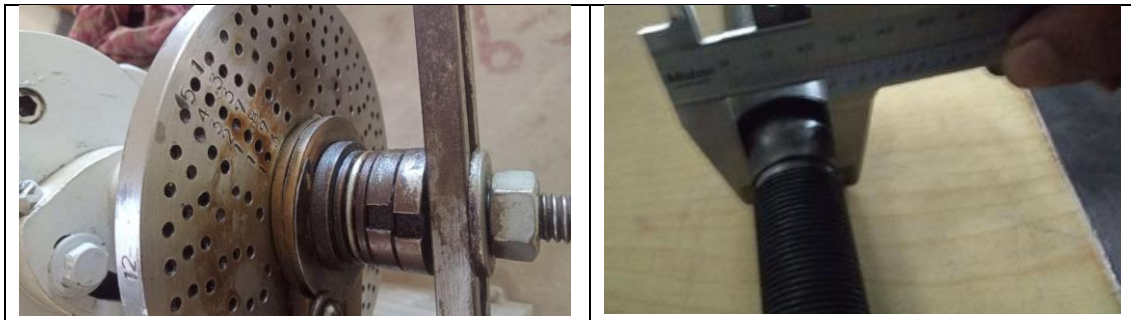
Fig. 4. Indexing and Arbor of the current Milling operation
