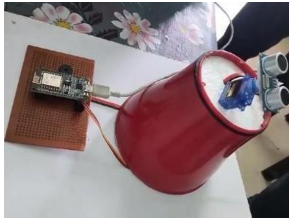
Fig.3. The smart sensor setup mounted on Servo motor.
