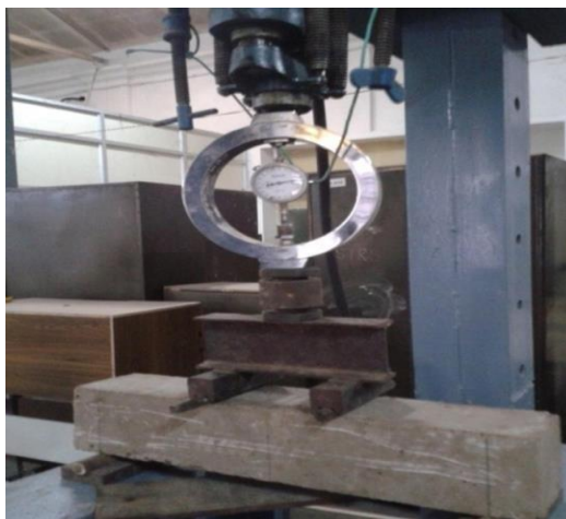
Figure 3.6 Test setup of flexural strength
