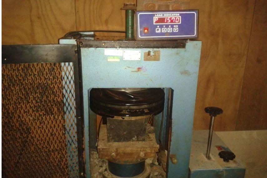
Figure 3.4 Test setup of compressive strength
