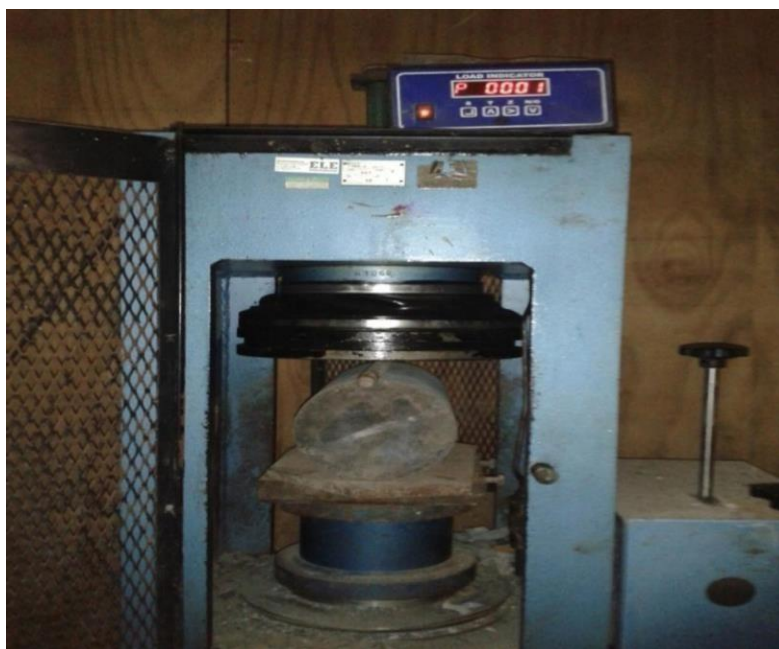
Figure 3.5 Test setup of split tensile strength
