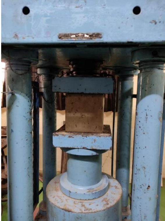
Figure 8: Cube specimen Test Setup
