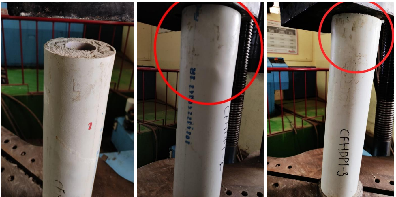
Figure 26: Deformation of CFDHPT-1, CFDHPT-2, CFDHPT-3
