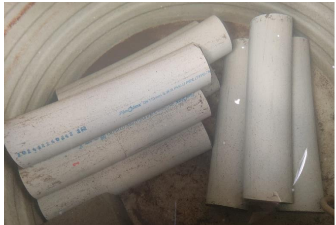
Figure 7: Curing of CFPT specimens
