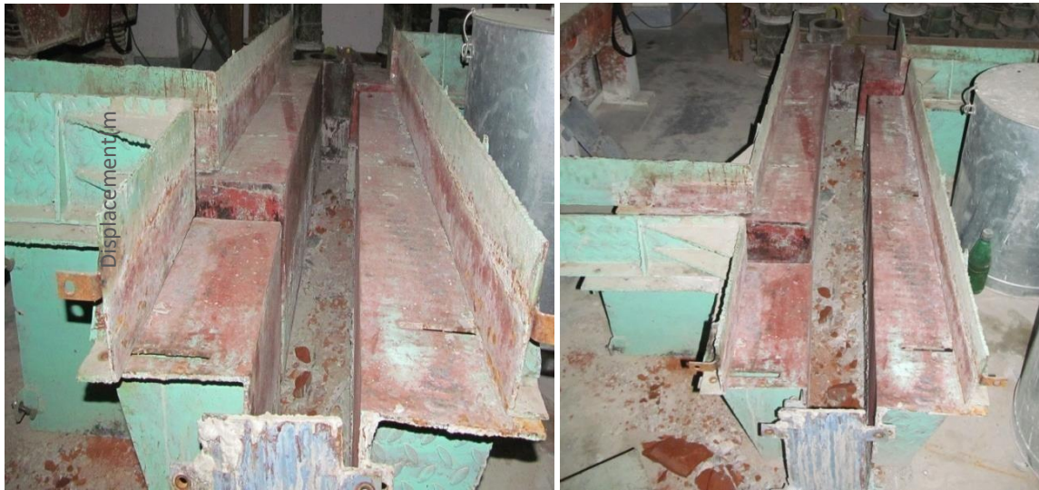
Figure 3-7. Steel Frame Used For Casting of RC T-Beam
