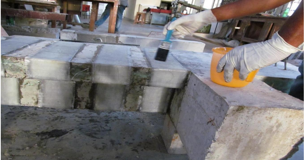
Fig. 3.5 Application of epoxy and hardener on the beam
