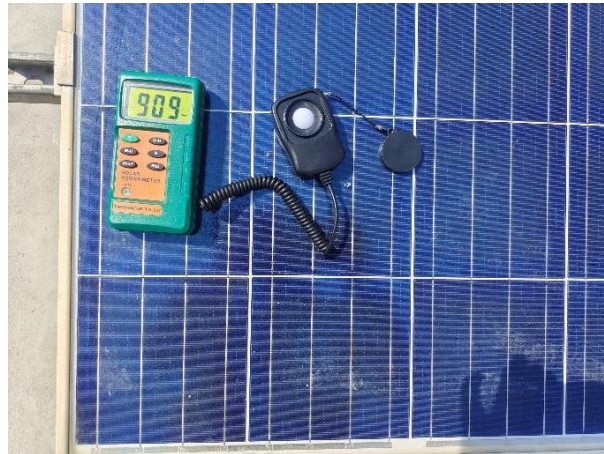
Fig. 3 Monofacial Solar Irradiance Measurement (Front)
