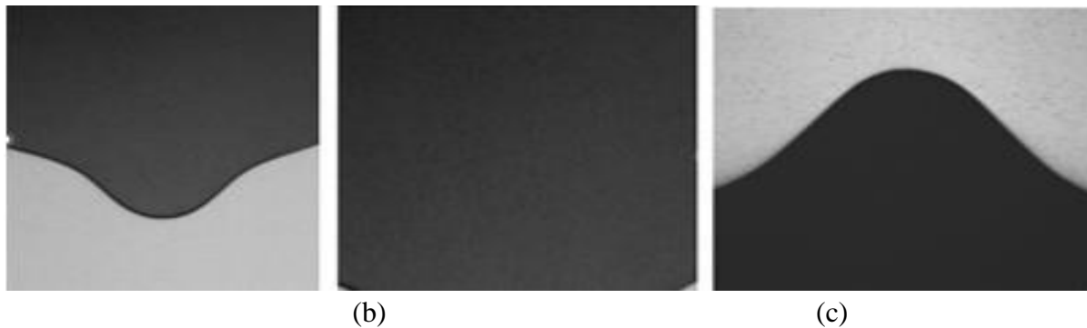
Fig-5 (a) the concave interface (initial growth), (b) the planar interface (middle growth), and the convex interface (end growth) along the VDS growth axis with increasing temperature (10-32)^{\circ}\text{C}
