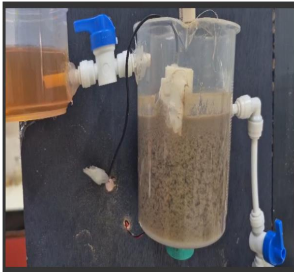
Figure C.5 (Chemical Coagulation): Sedimentation stage using Iron (III) Chloride ( \text{FeCl}_3 ) to precipitate suspended solid impurities from the raw greywater 5
