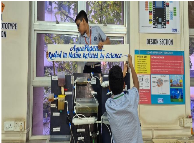
Figure C.3 (Apparatus): The complete 10-stage hybrid filtration prototype, integrating automated pumps, IoT sensors, and multi-stage filtration cartridges
