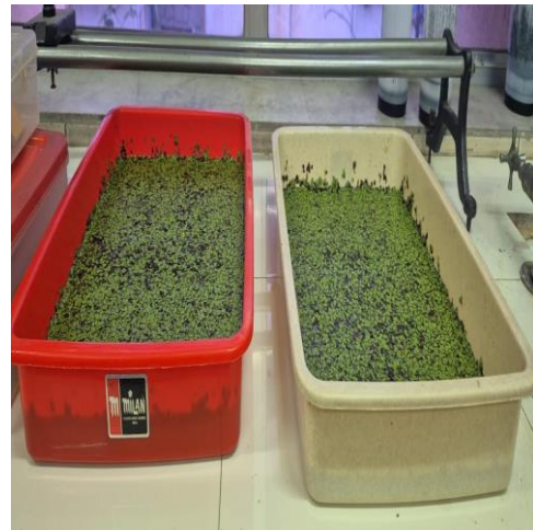
Figure C.4 (Rhizofiltration): Biological treatment tank utilizing Lemna minor (Duckweed) for the active absorption of nitrates, phosphates, and heavy metals.
