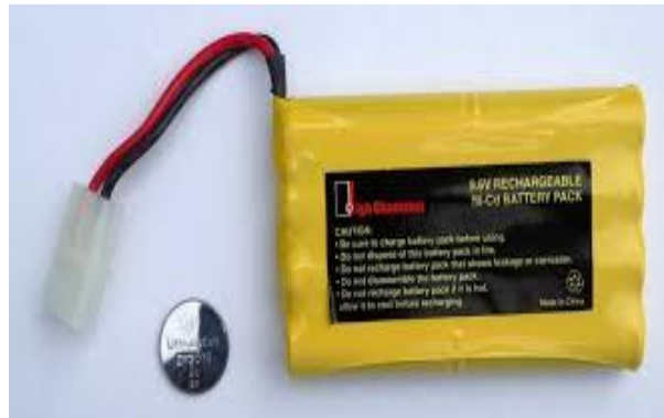
FIG 2: POWER SUPPLY (BATTERY)
