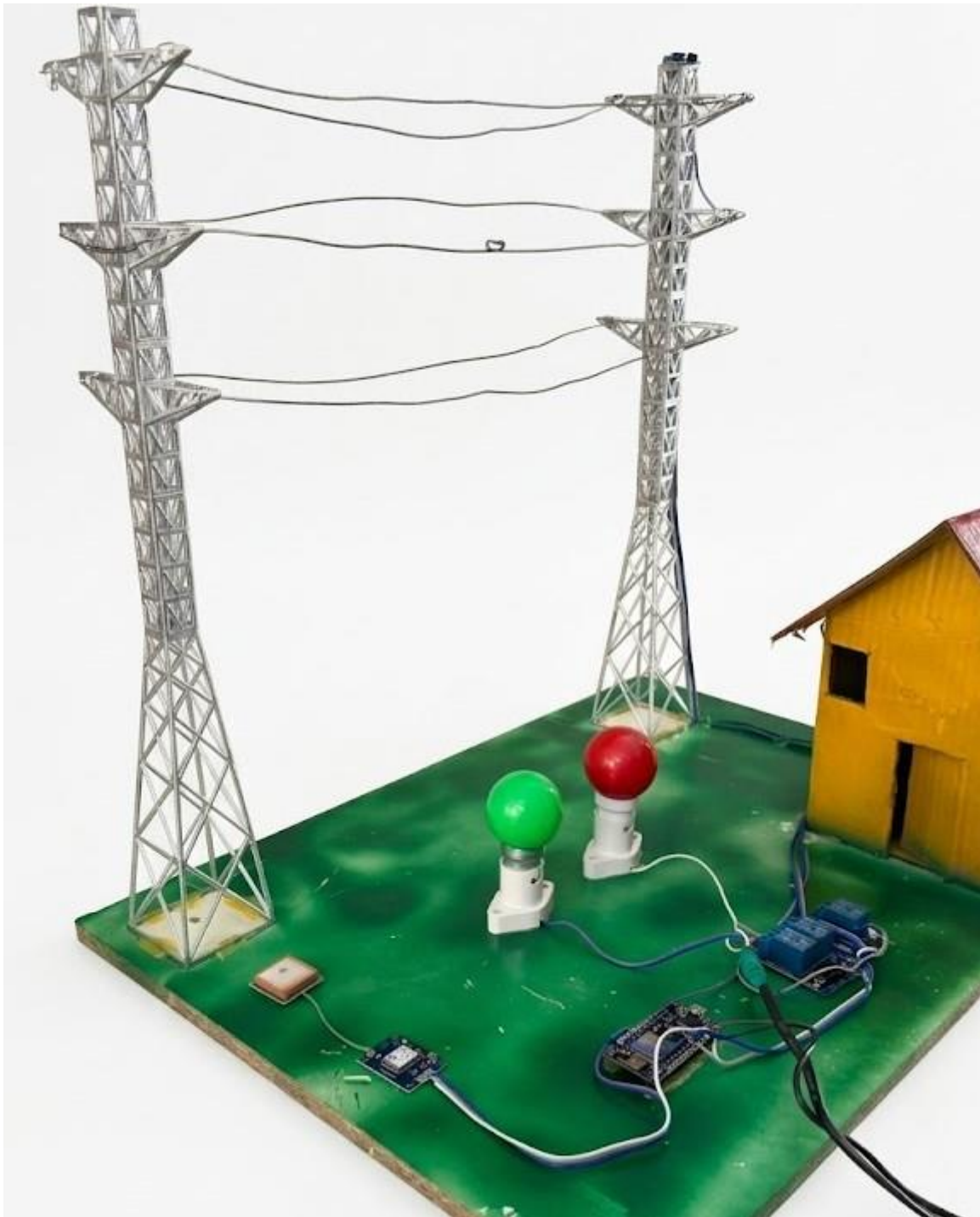
Fig. 2: Full Hardware Setup — NodeMCU, Sensors, NEO-M8M GPS Module & Wiring
