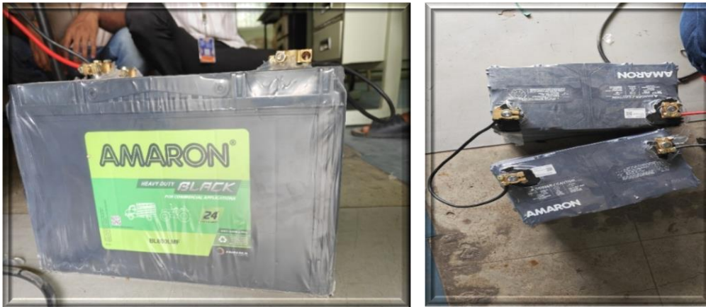
Figure 5.2.5: Lead-Acid Battery 12V,80Ah
