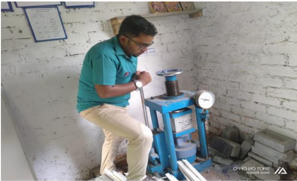
Plate-2: Compressive Strength Test
