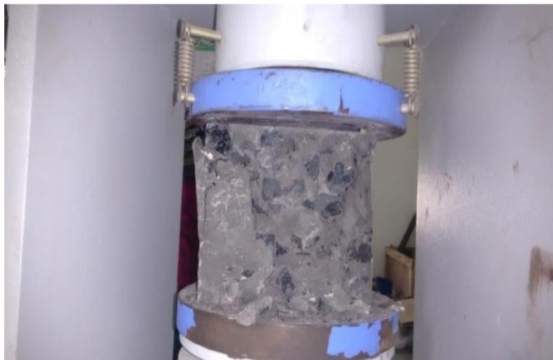
Fig: Compression Strength test set up
