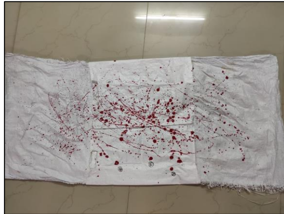
Figure 1 Long-shot view of simulated bloodstain pattern created using red acrylic paint on cloth, prepared under controlled laboratory conditions for LiDAR accuracy testing.
