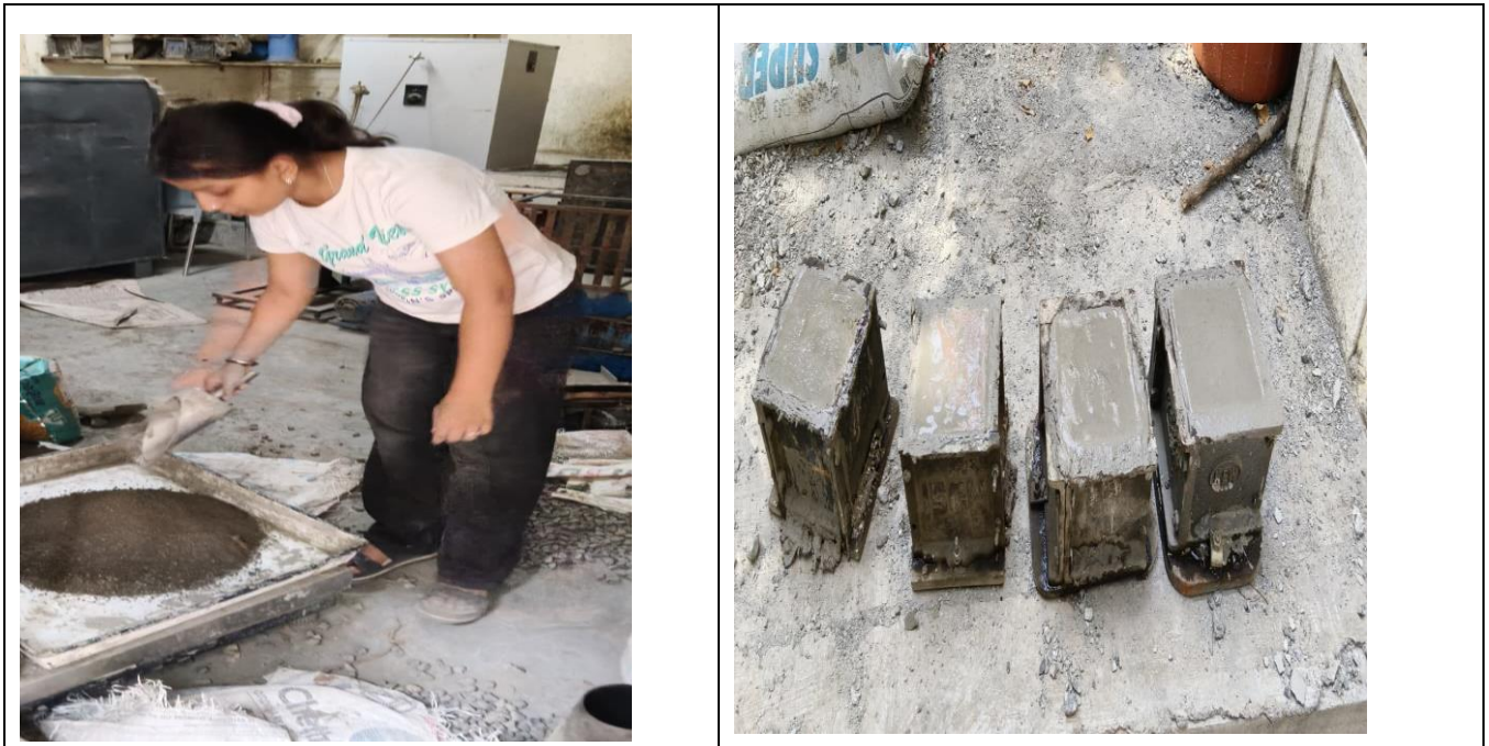
Figure 5: Demoulding and Water Curing
