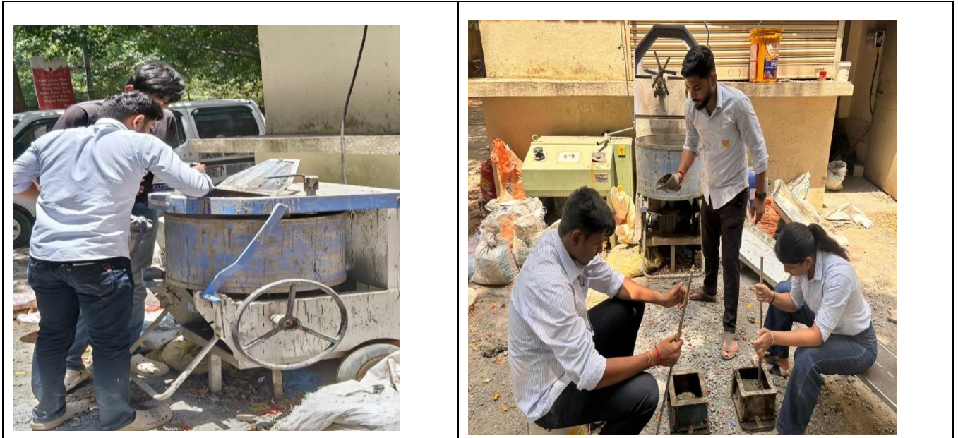
Figure 4: Casting of Concrete Cube Specimens
