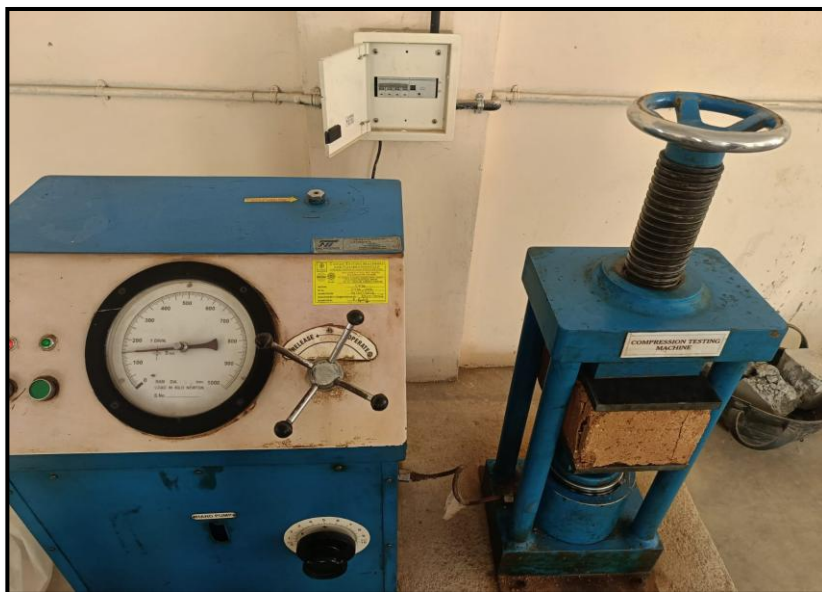
Figure 6: Obtaining maximum compressive strength from CTM machine
