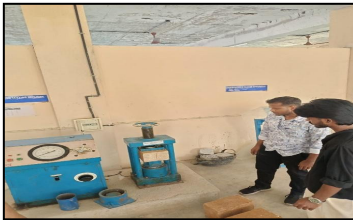
Figure 6: Obtaining maximum compressive strength from CTM machine
