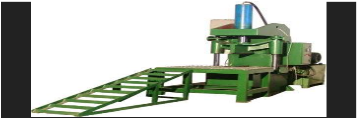
Fig.2.1 Rubber tire cutting machine (source: www.google.com/rubber tire cutting machine )
